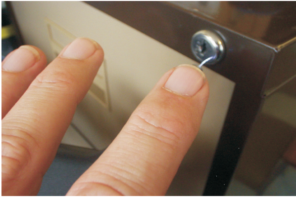
Captured on film! An electrostatic spark from a person's finger to a filing cabinet.
